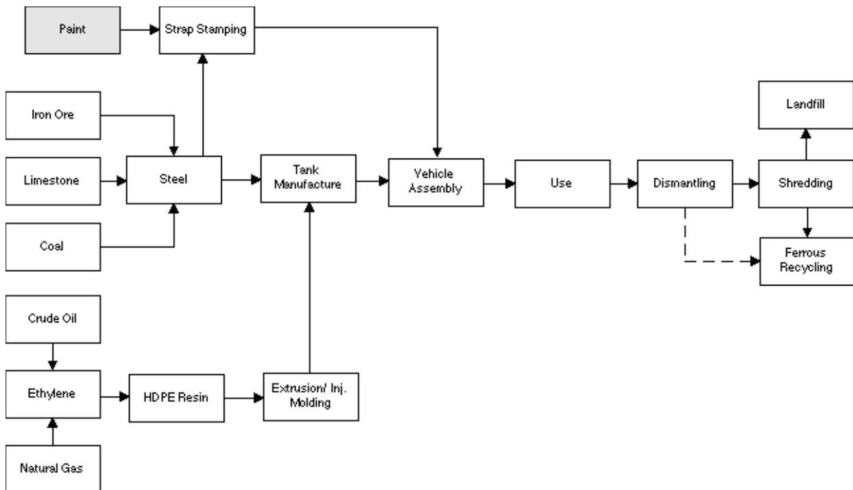
Figure 2. Steel Fuel Tank System Life Cycle
