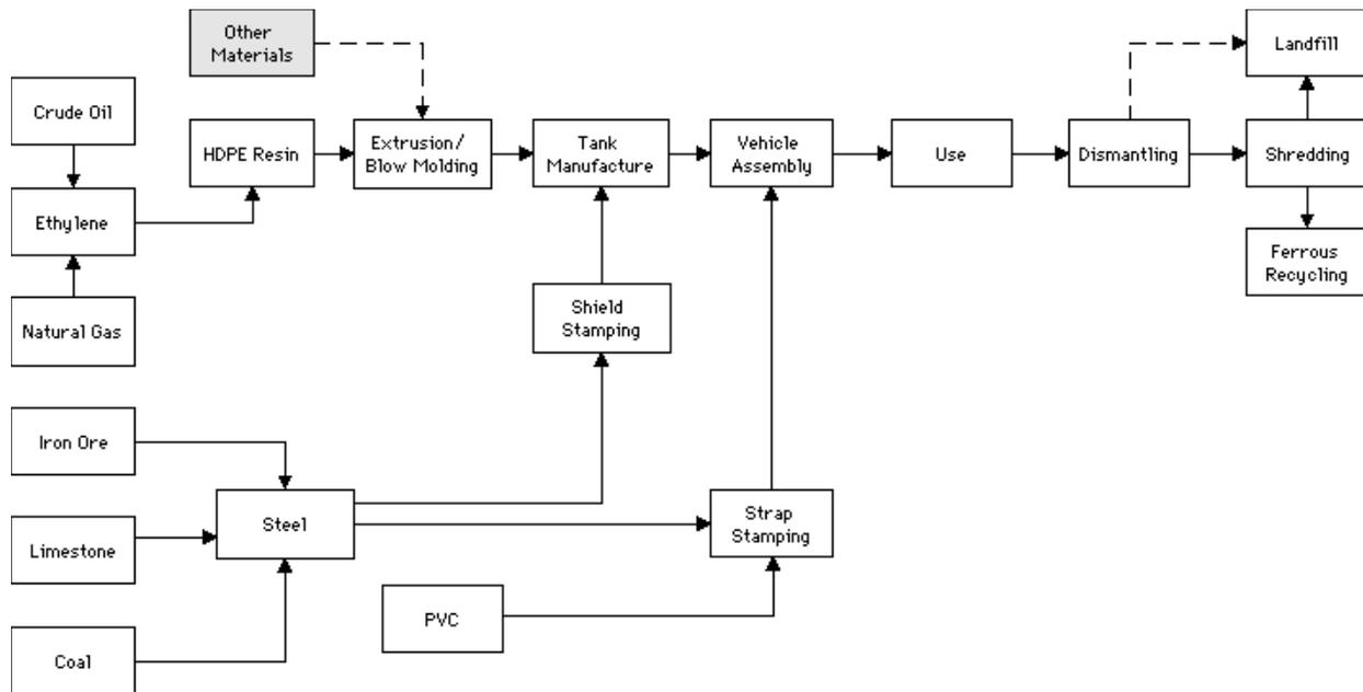
Figure 3. Plastic Fuel Tank System Life Cycle
