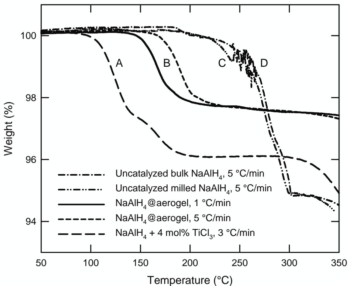
**Figure 3.** Thermogravimetric analysis (TGA) of four NaAlH<sub>4</sub> materials: A) ball-milled NaAlH<sub>4</sub> catalyzed with 4 mol% TiCl<sub>3</sub>, B) uncatalyzed NaAlH<sub>4</sub> melt-infused into 13 nm aerogel, C) uncatalyzed NaAlH<sub>4</sub> ball-milled for 5 hrs, and D) bulk uncatalyzed NaAlH<sub>4</sub>. The heating rates are specified in the legend. The NaAlH<sub>4</sub> content of the catalyzed sample is 90 wt%, while NaAlH<sub>4</sub>@aerogel is 48.6 wt% NaAlH<sub>4</sub>.
