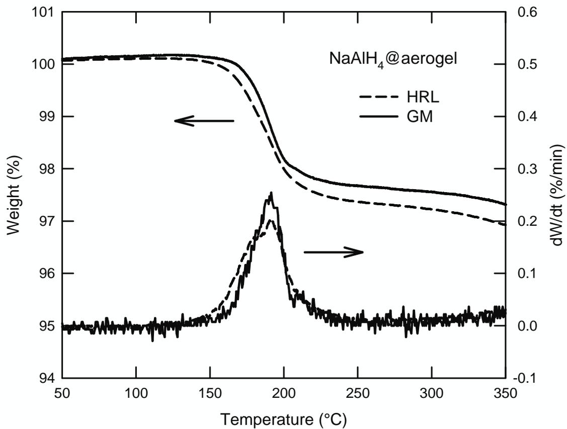
**Figure 5.** Thermogravimetric analysis (TGA) of the weight loss for two  $\text{NaAlH}_4$ @aerogel samples, one synthesized and measured at HRL and one at GM. Also shown is the first derivative of the weight loss showing the temperature at which the maximum rate of weight loss occurs.
