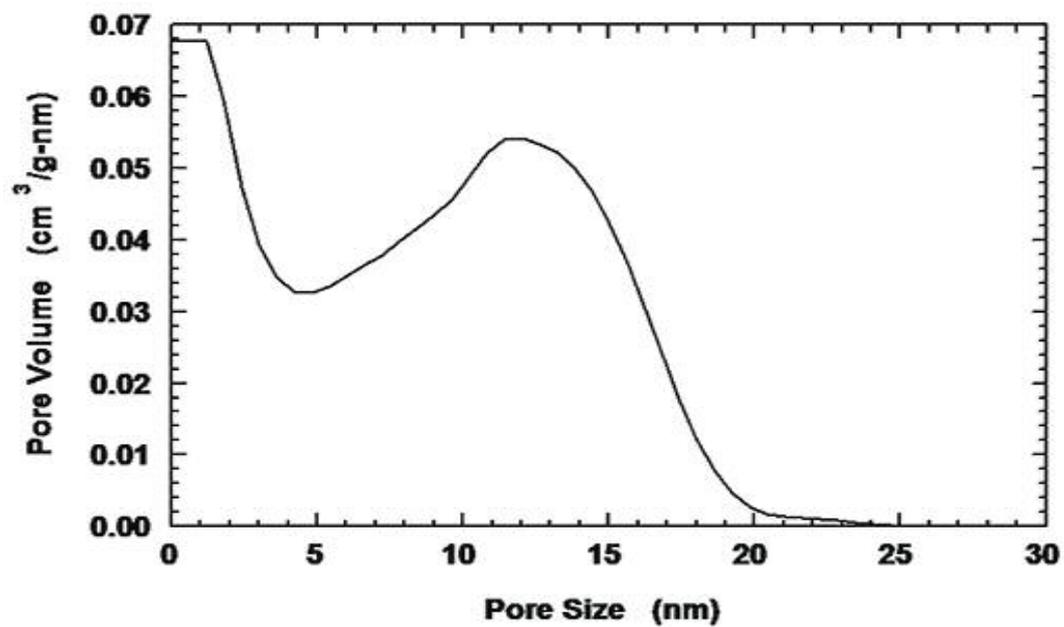
**Figure 1.** Pore size distribution of the carbon aerogel used in these experiments derived from an N<sub>2</sub> absorption isotherm.
